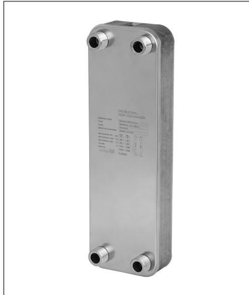
XBDW22 is double wall heat exchanger designed for application where the flow mediums are not allowed to mix. The double wall heat exchanger prevents primary media to be mixed with the secondary media if there is and internal leak in the unit.
